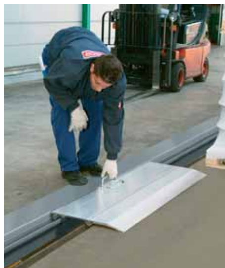
Ready for safe drive over.
